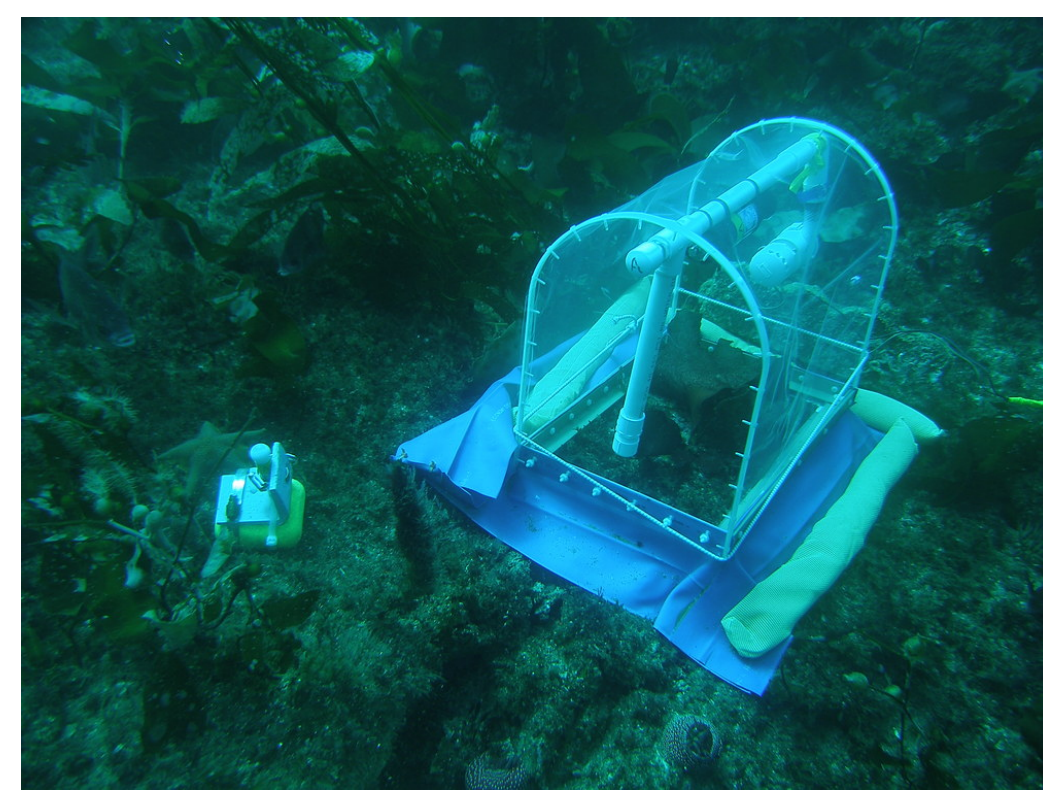
Above, a chamber for measuring in situ NPP in a benthic algal community at the Santa Barbara Coastal LTER.
