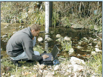
SBC researcher downloading data from stream gauge
