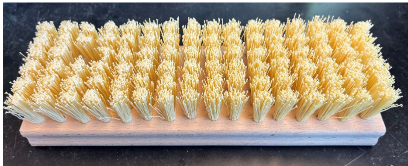
Figure 2. Wood-backed brush with polypropylene bristles measuring 20 x 7 cm (140 cm 2 ) used for recruitment sampling of invertebrates.
