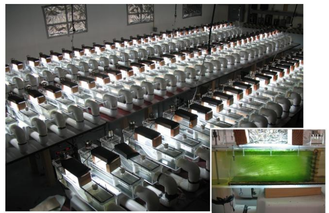
Fig 3. The environmentally controlled flume facility at UCSB houses 120 independently re-circulating stream channels where temperature, flow and light are all standardized. Each unit is fitted with an air-tight lid and a port for an O 2 probe that allows 1 o production to be estimated by gas exchange. A variety of algal species have been grown successfully in these flumes. The inset shows just one example of the filamentous alga Stigeoclonium growing in the 300-cm 2 working section of the channel.
